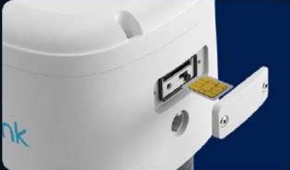
1. Insert a nano SIM card and turn on the camera.
